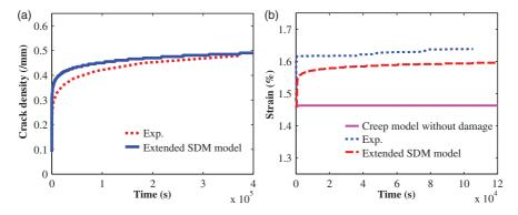
**Figure 8.** Predicted and experimental (Ogi and Takao, 1999) results for a  $[0/90_3]_s$  cross-ply laminate subjected to a constant creep stress of 530 MPa: (a) 90° ply crack density evolution and (b) corresponding laminate creep strain.
