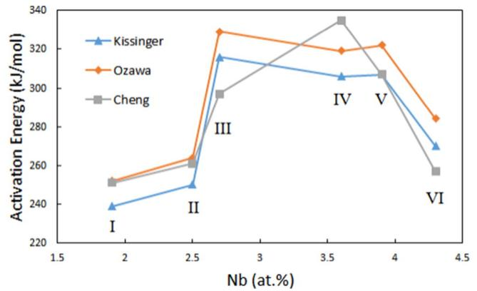
Fig. 8. Comparison of activation energy found through Kissinger, Ozawa and Cheng analysis with increasing Nb content (Compositions I–VI given in Table 1).
