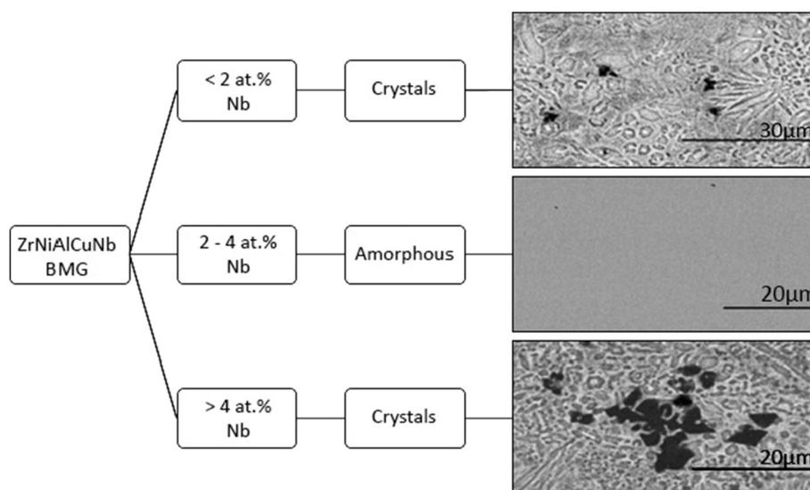
Fig. 3. Effect of Nb concentration on the crystallization behavior noted in XRD, showing a high GFA range from 2 to 4 at.% Nb.
