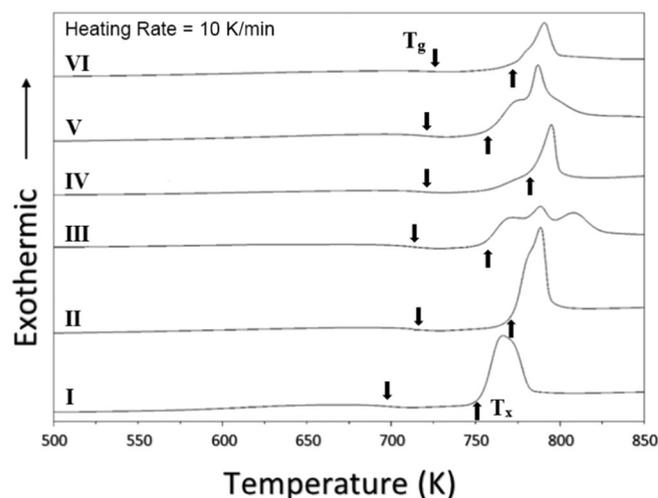
Fig. 4. DSC comparison for all as-cast samples at a heating rate of 10 K/min.
