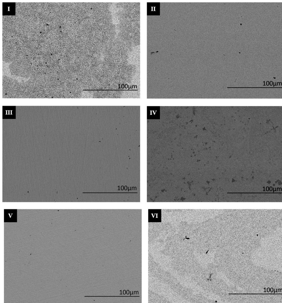
Fig. 2. SEM micrographs for cross-sections for as-cast rods taken at 500× magnification to compare crystalline features. Samples I, IV and VI show clear dendritic crystal formation. Samples II, III and V do not show any indication of crystals; however, XRD indicates oxides are present in Sample II that cannot be seen in SEM.
