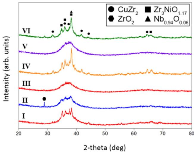
Fig. 1. XRD patterns taken for all as-cast samples (Compositions for I–VI given in Table 1).
