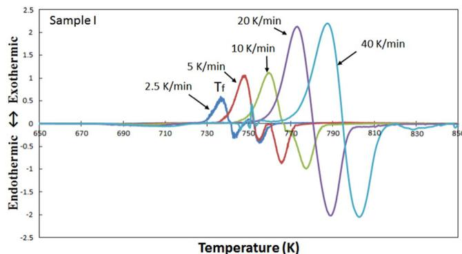
Fig. 7. Example of the DDSC curves for Sample I used to find  $T_f$ .
