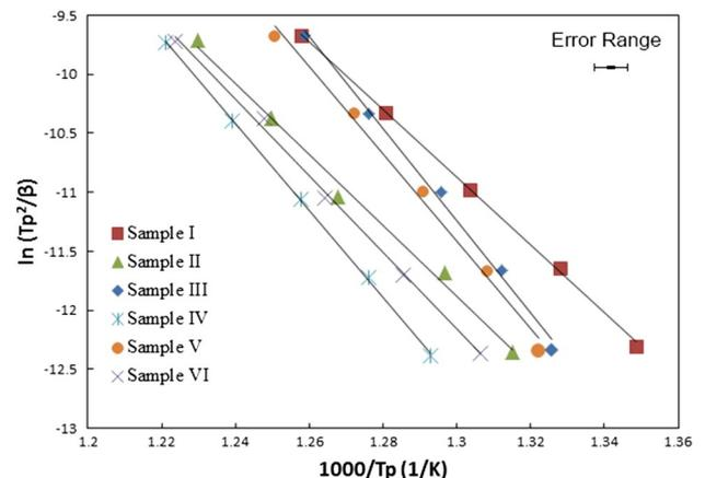
Fig. 6. Kissinger plot for suction cast 3 mm diameter rods of Zr-Ni-Al-Cu-Nb alloys using peak temperature of the first crystallization peak. Error range is shown in the top right corner. (Compositions I-VI as shown in Table 1).
