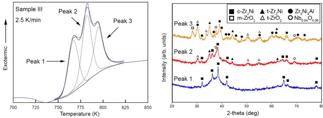
Fig. 5. Deconvoluted crystallization peaks for Sample III at a heating rate of 2.5 K/min with corresponding XRD scans to identify existing phases at each peak step.
