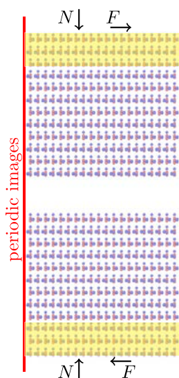
Fig. 6. Ice Friction Model for Problem (C) as defined in Section 4.3: two slabs of ice will be brought into contact by applying normal and friction force by harmonically restricting the molecules in yellow indicated areas. Red lines indicate periodic box boundaries. (For interpretation of the references to color in this figure legend, the reader is referred to the web version of this article.)
