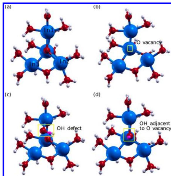
**Figure 1.** Optimized geometric structures of (a) pristine  $\text{In}_2\text{O}_3$ , (b)  $\text{In}_2\text{O}_{3-x}$ , (c)  $\text{In}_2\text{O}_3(\text{OH})_y$ , and (d)  $\text{In}_2\text{O}_{3-x}(\text{OH})_y$  surfaces in the ground state. Indium atoms are represented in blue, hydrogen saturators in white, oxygen atoms in red and the hydrogen atom of the surface OH group in pink.
