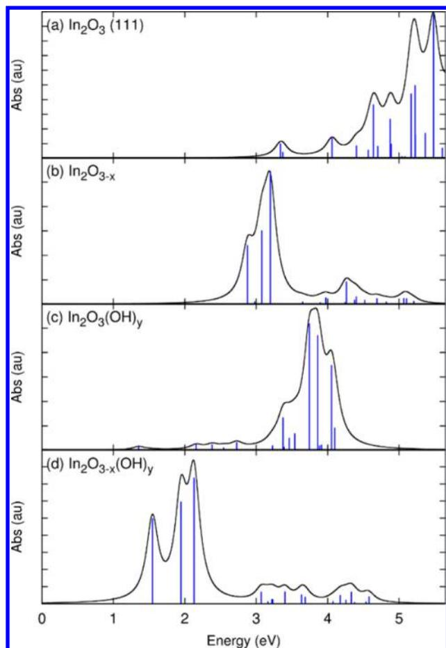
**Figure 2.** TDDFT-calculated absorption spectra for (a) pristine  $\text{In}_2\text{O}_3$  and defected (b)  $\text{In}_2\text{O}_{3-x}$  (c)  $\text{In}_2\text{O}_3(\text{OH})_y$  and (d)  $\text{In}_2\text{O}_{3-x}(\text{OH})_y$  surfaces. Vertical lines correspond to unbroader excitation energies and oscillator strengths.
